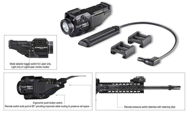
Material/Lens 6000 Series machined aircraft aluminum with Type II Mil-Spec anodized finish. Switch housing: Impact and chemical resistant engineered polymer. High temperature, shock mounted, AR coated, impact resistant Borofloat<sup>®</sup> glass.
